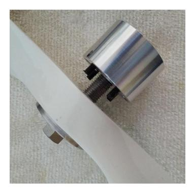
Press the prop hub onto the studs by tightening the M10 titanium bolt onto the hub and the hub onto he studs.
