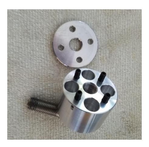
Slide the titanium center bolt through the 3mm aluminum prop washer and through the propeller's shaft bore hole.
