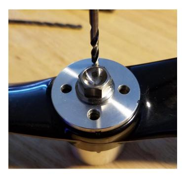
Place one of the 4mm bolts into the partially drilled hole to keep the prop washer from moving, and continue to drill the rest of the hole, using the bolts in each hole as you go along.
