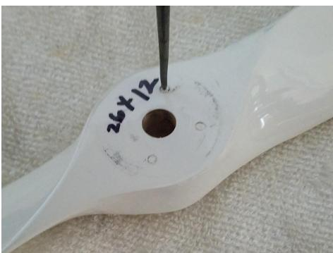
Mount the prop onto the spacer with the titanium bolt.
