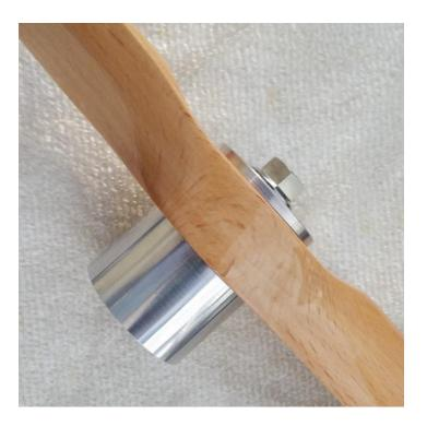
Making sure the bolt holes are aligned as needed to fit the spinner prop blade openings, mark the spacer, prop hub, and prop washer.
