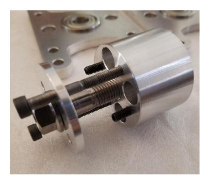
The second option is just two studs with the center bolt, or you can use 4 studs as well.
