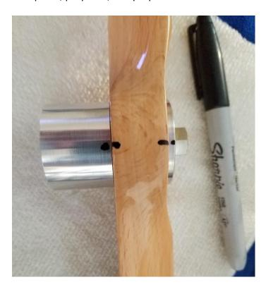
Drill one hole at a time halfway through the hub.
