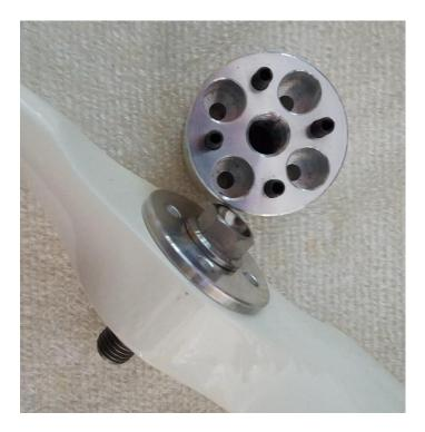
Thread the M10 titanium bolt onto the spacer.
