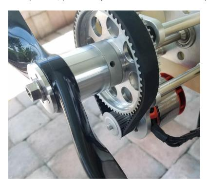
Important – With all options, please make sure that the titanium center bolt is seated flush on the aluminum prop washer. There is a ridge under the titanium bolt head flange and the flange will not seat flush on the prop washer unless it is tightened enough to press the flange flush the first time you mount a propeller. You may need to do this with both sides of the prop washer if you do not use the same side against the flange all the time.
