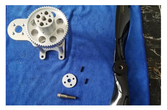
Hand thread the setscrews into the M4 holes in the StinGR hub with the pointed ends exposed.
