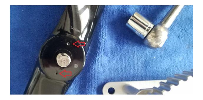
Use a small drill bit to start the hole so that the larger bit doesn't "walk" along the slick carbon finish.
