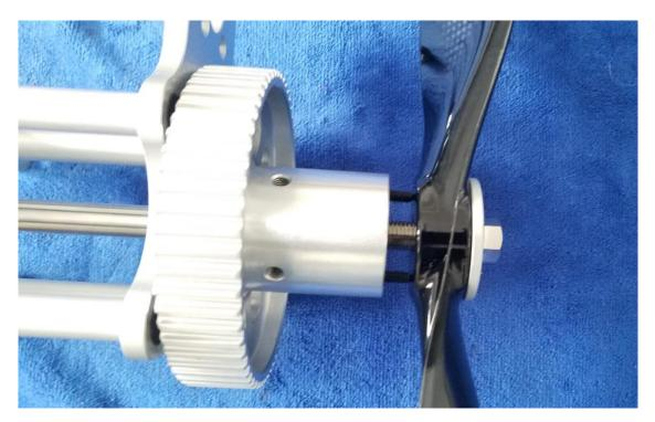
Tighten the M10 bolt so that the prop hub on is forced onto the setscrew points tight enough to assure that a mark is made by the setscrew points on the propeller hub.
